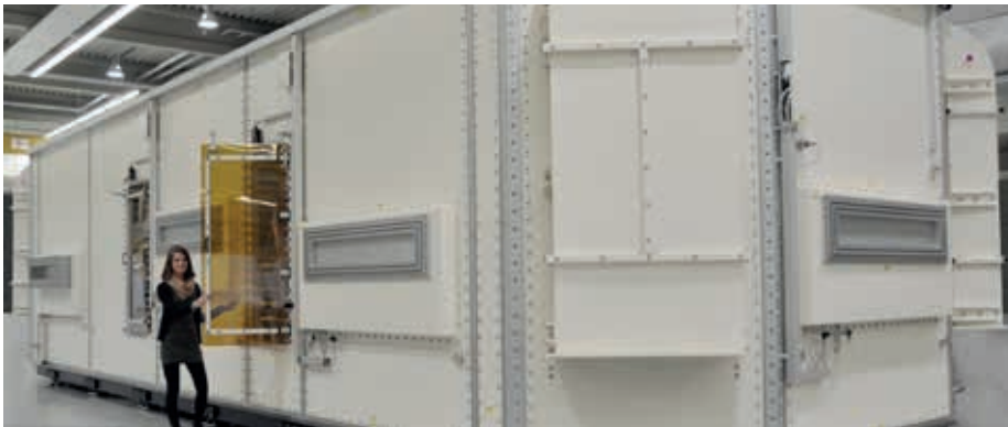
Large enclosure operating under inert atmosphere ( O_2 and H_2O < 1 ppm) combined with a clean zone (ISO Class 2)
